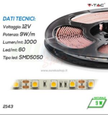
STRISCIA LED 12V 9W NATURALE 4500K 1000LM 60LED/MT SMD5050 IP20
