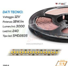
STRISCIA LED 12V 18W CALDA 3000K 3000LM 240LED/MT SMD2835 IP20
